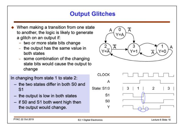
Let us examine the state machines output Y in detail. When we transit from state 1 to state 2, it is possible that we pass through state 0 for a very short time. This is because when S1:0 = 01 moves to S1:0 = 10, S1 could be slightly slower than S0 in the transition. Hence S1:0 = 00 occurs temporarily.
