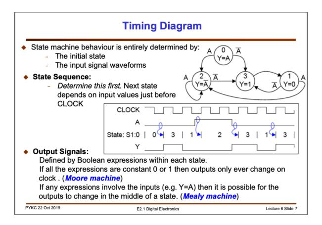
It is important to note that the behaviour of a FSM is determined by the initial state. Given the state diagram and the initial state (assumed here to be state 0), and waveform of the input A, we can easily trace the subsequent states S1:0 and the output Y.
