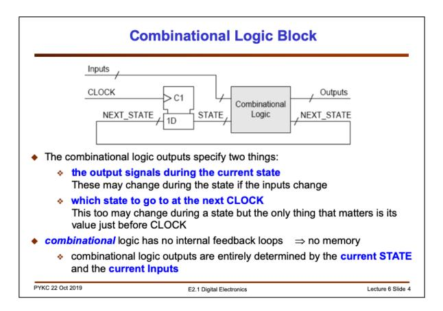
The combinational logic circuit in a FSM performs two separate tasks:
