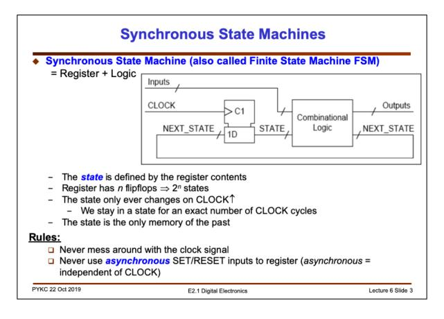
Here is a simplified generic diagram of a finite (or synchronous) state machine (FSM or SSM). A set of D-flipflips are used to store the current state value. The current state together with external inputs are fed to a combinational logic circuit to evaluate two things: the **next state** and the **current outputs**.
