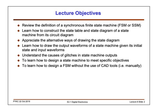
In the previous lecture, we examined how to use counters and shift registers to produce arbitrary digital signals that could be used as control signals to a digital system. While such circuits could be fast (particularly with shift registers), the design process is not systematic. For complicated control logic, it is far better to design such circuit as a synchronous (or finite) state machine.
