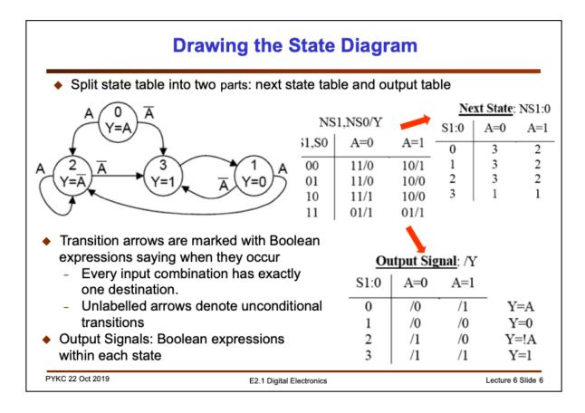
Another very powerful tool to show the function of a FSM is to use state diagram (one that uses "bubbles"). For clarity, let us split the state transition table into two tables: one for next state NS1:0, and another for the output signal Y.
