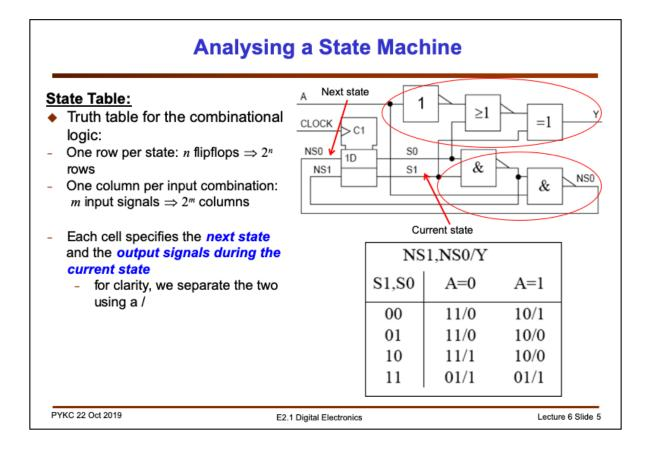
Shown here is a simple FSM in details. The upper group of gates are used to compute the output signal Y. The lower group of gates are used to work out the next state values NSO and NS1.
